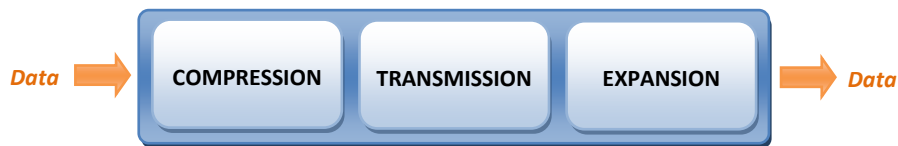
Figure 6: Functional architecture - Data Transmission block
