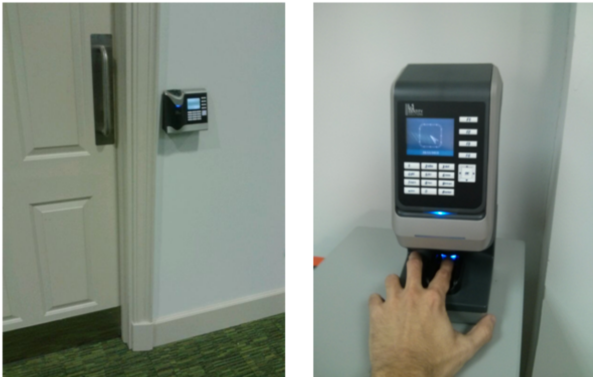
Figure 4. Finger print recognition device and finger vein recognition device
